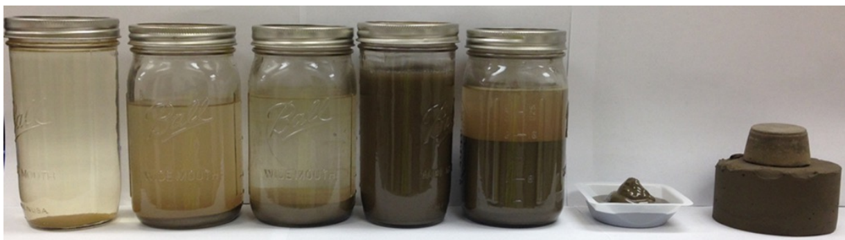
Figure 3. Progression of FGD Wastewater to Solidified Residual
