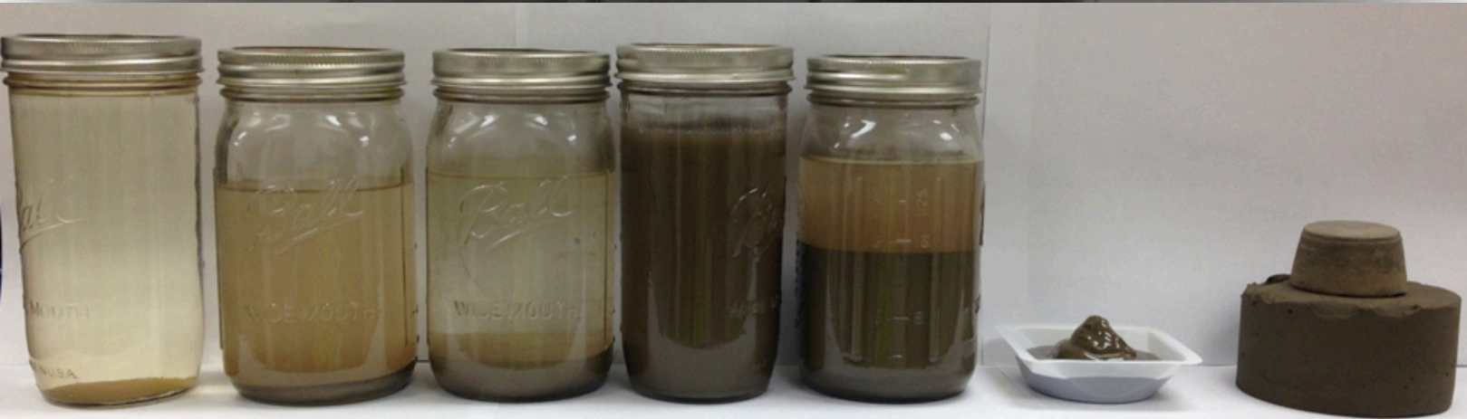
Figure 3. Progression of FGD purge water in the Heartland Concentrator from raw feed to solidified and stabilized residual.
